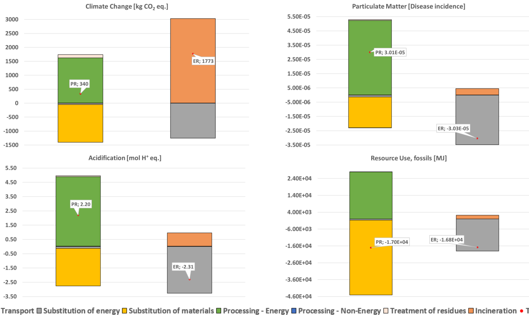
Figure 9. Management of 1 tonne of EPS construction and demolition waste through physical recycling (PR: solvent-based separation/dissolution and subsequent PS granulate production) and energy recovery (ER: incineration): Climate Change, Particulate Matter, Acidification, and Resource Use, fossils impact indicators. Negative values represent savings, while positive ones represent burdens. See Table 1 for a description of the different treatment scenarios and technologies.
